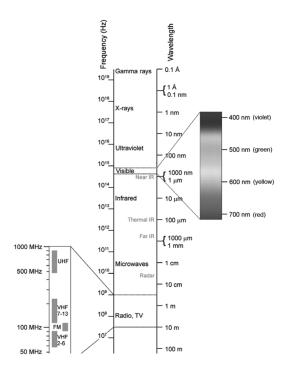
The diagram shows, in three columns, different sections of the electromagnetic spectrum. The far left column shows the radio and television waves portion of the electromagnetic spectrum. The central column shows all the types of waves in the electromagnetic spectrum. The far right column shows the visible portion of the electromagnetic spectrum.
